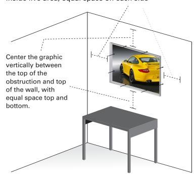
If both Type #1 and Type #2 are in same room or hallway, the vertical center of ALL graphics should be height of Type #2
